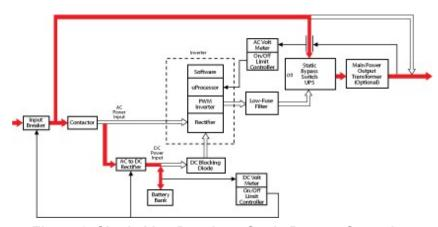
Figure 2 Single Line Drawing - Static Bypass Operation
