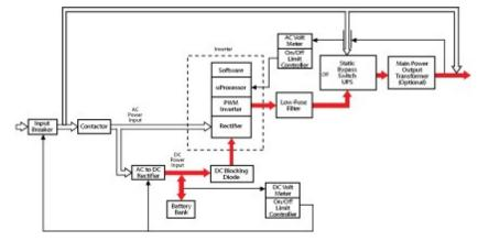
Figure 3 Single Line Drawings -AC Loss/Battery Operation
