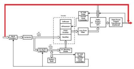
Figure 4 Single Line Drawings –External Maintenance Bypass Operation
