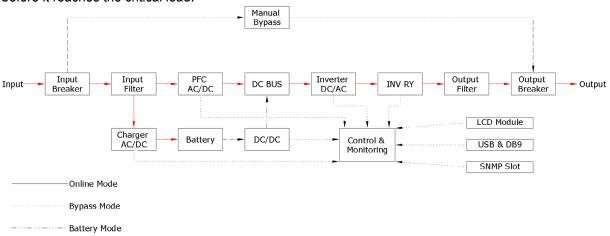
Figure 2 Single Line Drawing - Normal Operation
