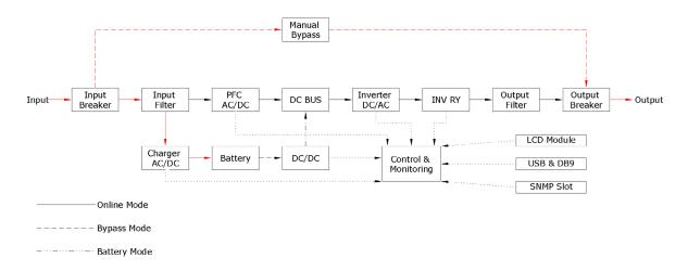
Figure 3 Single Line Drawing - Static Bypass Operation
