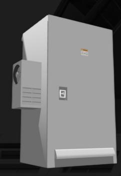
Extreme power factor rated. Made to handle elevators starting and stopping when batteries are the only source of power. The LP3 is designed to absorb elevator regeneration energy when operating on battery power during a utility outage without adding other equipment. Under normal operation, when the utility power is available, the regeneration energy is absorbed in the normal building loads.
