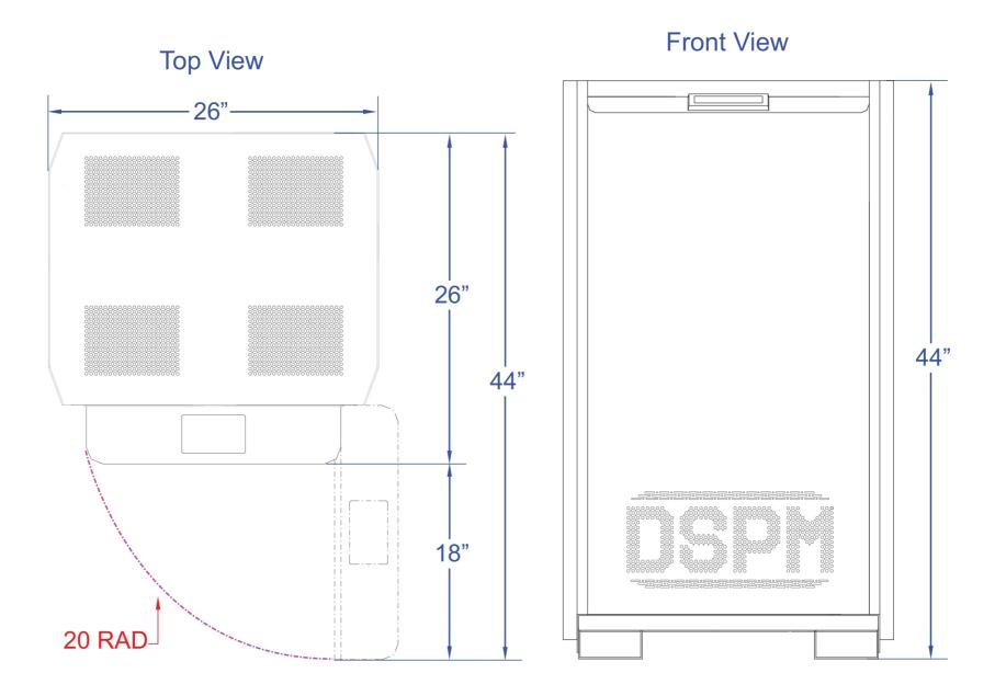
Per code requirements please leave 3" on each side of the cabinet including the back, and a 3 foot clearance in front.
