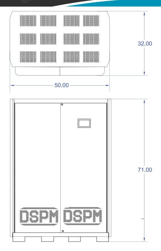
Per code requirements please leave 3" on each side of the cabinet including the back, and a 3 foot clearance in front.
