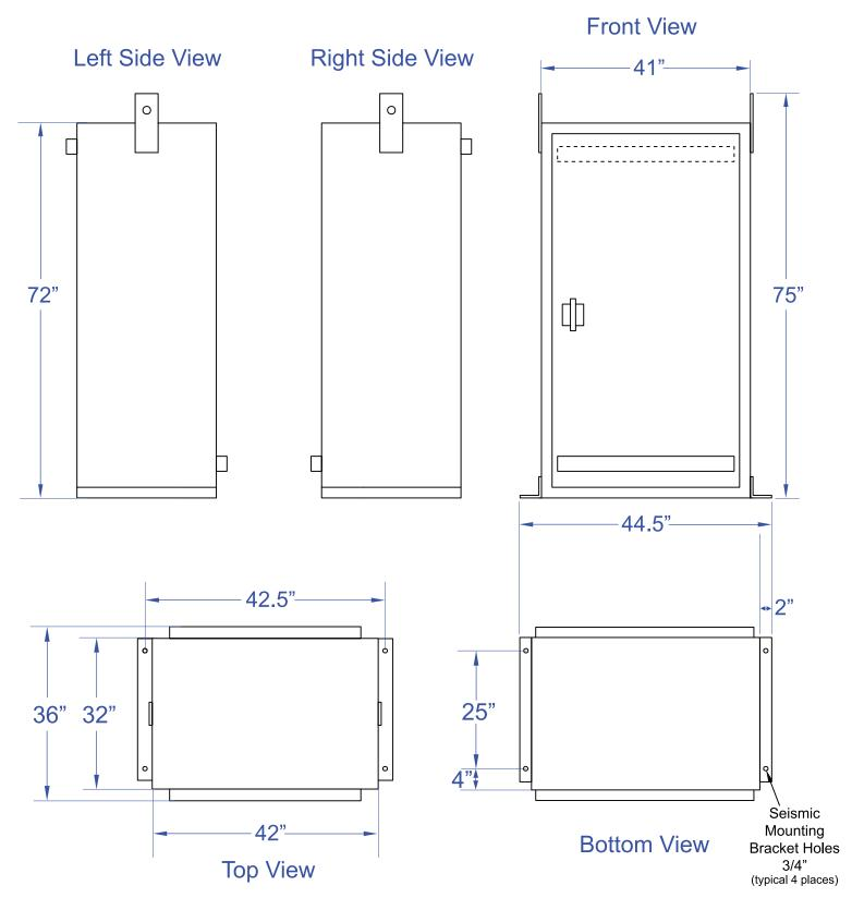
Per code requirements please leave 3" on each side of the cabinet including the back, and a 3 foot clearance in front.
