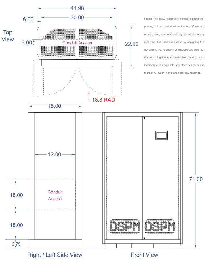
\*Contact factory for special conduit access arrangements
